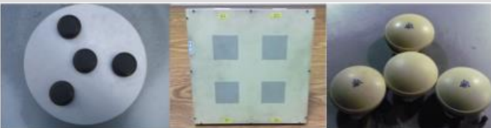
Controlled reception pattern antenna (CRPA) receiver & data collector developed by Y.H. Chen
